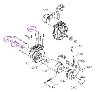
Replace the driver wheel by the following steps if it is worn out or deformed. Remove the cap(5.62) and follow preceding step above.
