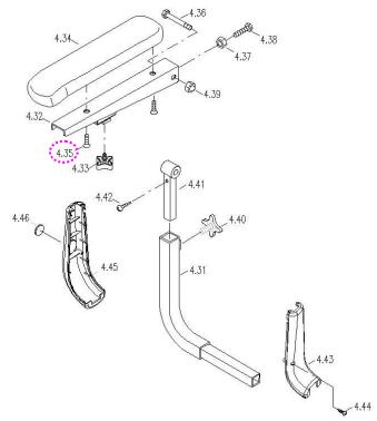
Note: The arm tube protective shrouds (4.43 and 4.45) are option parts for powerchair.
